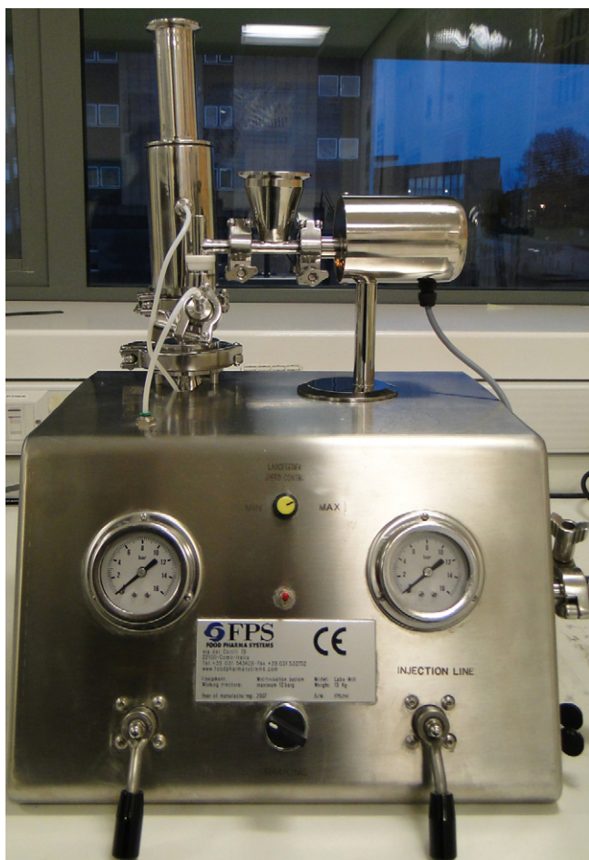
Fig. 1. The spiral jetmill (FPS, Italy).
